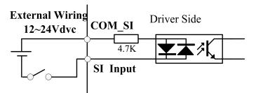
**A.** The power supply is provided by user, DC 12-24V, current  $\geq$ 100mA, if the power polarity connects reversely, the drive won't run.
