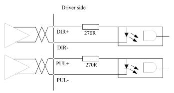
Wiring method of 5V differential signal (Pin 3/4/5/6)
