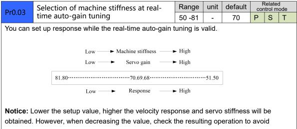
oscillation or vibration. Control gain is updated while the motor is stopped. If the motor can't be stopped due to
